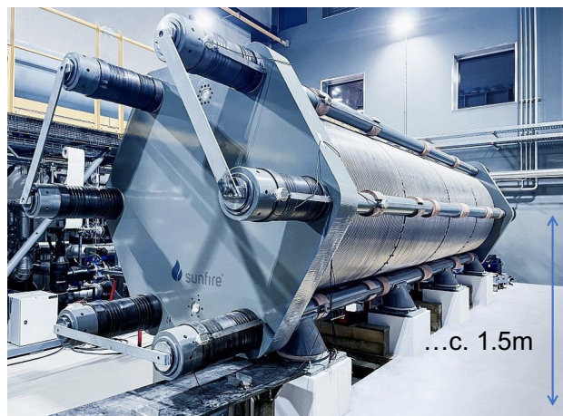
...the plates are formed into ‘stacks’...photo is 10MW Alkaline electrolyser stack (AEL)
